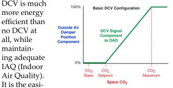
est DCV method to configure. However, where VOCs, radon, or other pollutants become excessive during unoccupied times (with no ventilation), the FlexStat's Standard or Advanced DCV configuration is recommended.
