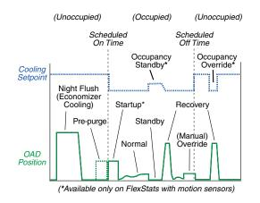
For more details about DCV configuration and operation, see the **FlexStat Operation Guide** and **FlexStat Application Guide**.
