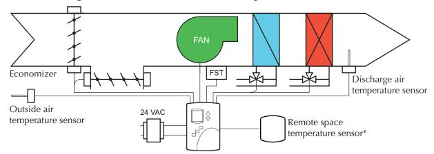
\* Economizer, fan status switch, discharge air and remote space temperature sensors are optional items.
