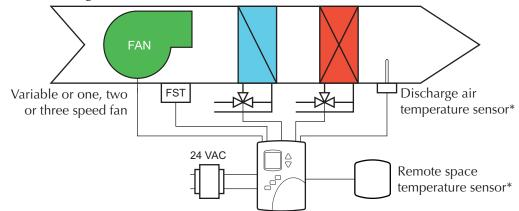
\*Fan status switch, discharge air and remote space temperature sensors are optional items.
